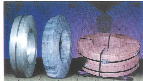
PACKING : The finished material is oiled with rust preventives and packed in Hessian Polyhessian, VCI papers and palletized as per the customer's requirements.
